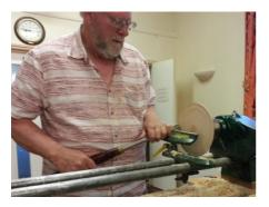
Now start in the centre to dig in, working back towards the outside with each successive cut. Don't take the centre too deep at this stage before finishing the outside edge.
