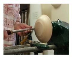
When the edge is trued up, move the toolrest round to the base. Make sure it's square to the wood to make the cuts easier.
